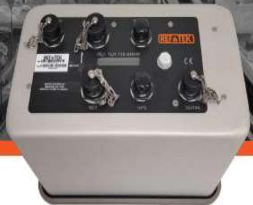
The 130-SMHR Strong Motion Accelerographs provide accurate and timely data and information for seismic events, including their effects on buildings and structures by employing modern monitoring methods and technologies. Both models are made for continuous monitoring of earthquakes and other seismic events, and the recording of strong earthquake shaking at ground sites, in buildings and critical structures.
